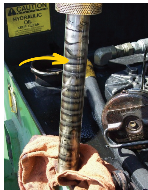
Millions of steel particles extracted from hydraulic fluid by a FilterMag™ reservoir magnet.
